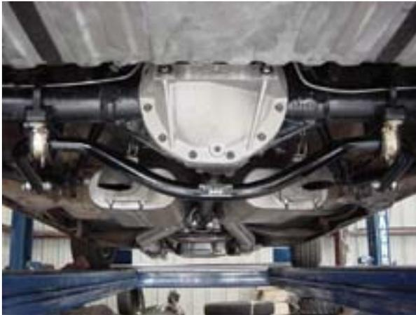
3.73 GM 12 bolt with welded tubes &
