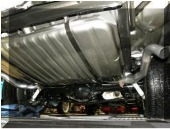
body was done on a rotisserie and the decision was made to paint the bottom of the car. Normally the car would be chassis black, but I also decided to paint the engine compartment and trunk in the body colour. My reason for this, was the fact that it is much easier to keep the car clean. The car is painted the original colour, Antique Metallic Pewter. The car has the original 396
