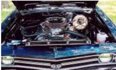
It now sports a TH 400 transmission with a few upgrades. The engine of choice was a 427 incher. All engine parts were new with the exception of the block and heads. Compression ended up at 10 to 1 with 450 horsepower and 499 pounds-feet of torque.
