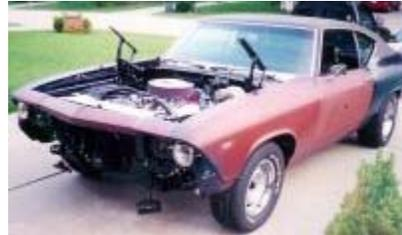
While the interior was out, the doors, trunk and behind dash were painted with rust resistant paint. Over the next three years the body was slowly completed including an original fender, SS hood and grill. During this time various engine and tranny parts were being attained.
